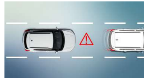
Front Vehicle Start Warning (FVSW) FVSW attracts the driver's attention with a visual pop-up alert and audible sound when the vehicle directly in front starts to pull away.
