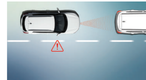
Safety Distance Warning (SDW) SDW calculates the distance to the vehicle in front and warns the driver when a safe distance is not maintained.
