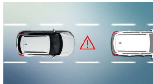
Forward Collision Warning (FCW) Alerts the driver when another vehicle or pedestrian appears in the path of the vehicle.
