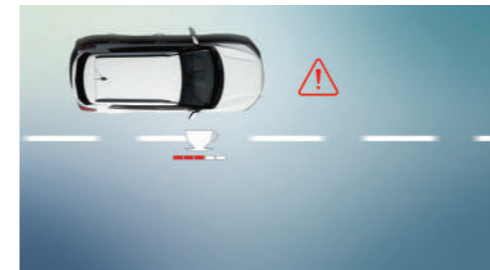
Driver Attention Warning (DAW) If the DAW system senses the driver's attention level has been significantly reduced, it gives an audible warning and a graphic on the cluster.
