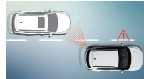
Blind Spot-detection Warning (BSW) Automatically assists braking if there is a risk of collision with vehicles in the blind-spot while changing lanes.
