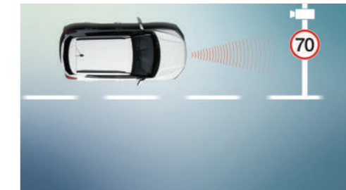
Traffic Sign Recognition (TSR) This recognises traffic signs and relays the information displayed on the sign to the driver through the cluster.
