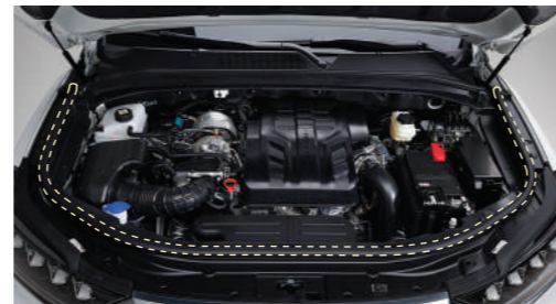
Engine room around sealing cover
